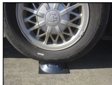
Park a vehicle wheel on top of the base for 15 seconds.
