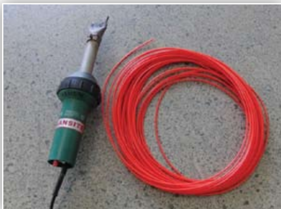
Welder & HDPE Plastic Wire
