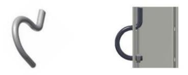
Figure 5 Placement of the Cable Lock Bolt
