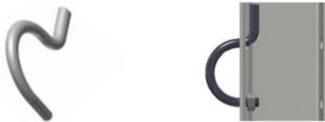
Figure 5 Placement of the Cable Lock Bolt
