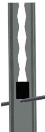
Figure 11 1 st Cable Installed
