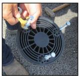
Step 4: Assemble the screws and anchors onto the base and tighten with wrenches.
