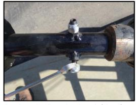
Step 1: Place the guide collar tool on the end of the Safe-Hit SHTOL-30-6-X manual driver tool stem. Tighten the two set screws and then secure with the locking nuts.
