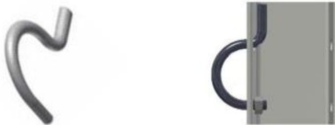
Figure 6 Placement of the Cable Lock Bolt
