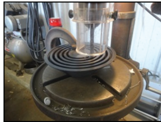
Use 25/64" drill to complete starter holes in base bottom.
