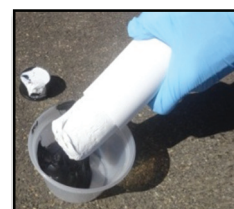
Use mixing stick to push epoxy into container. Thoroughly mix both parts to a solid gray consistency with no black or white streaks.
