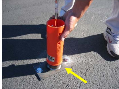
Step 6: Align the hinge tube index mark and torque the 1/2" bolt [30 ft-lb].
