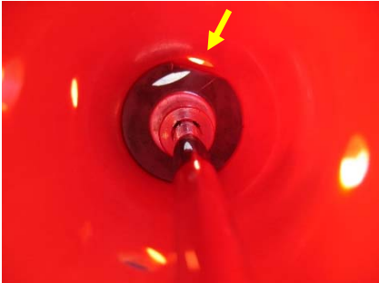
View looking inside the hinge tube. Flat is lined up with the hole.
