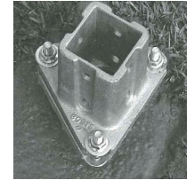
S-Q 8 Casting with 2.5" square perforated galvanized post and Cast Base.
