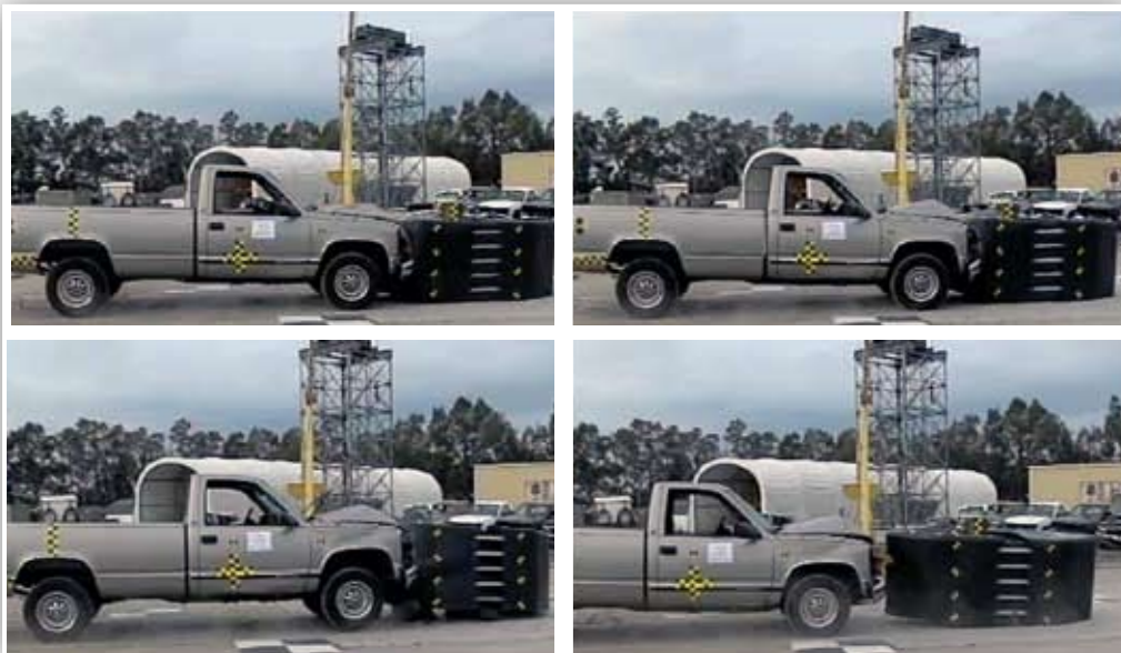
2000kg Pick-up truck impacting head-on with a pole using the RAPTOR™ at 31mph (50kph)
