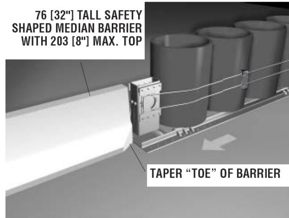
Figure 10 REACT 350® Narrow (36") with Self-Contained Backup Shielding Safety Shape Barrier
