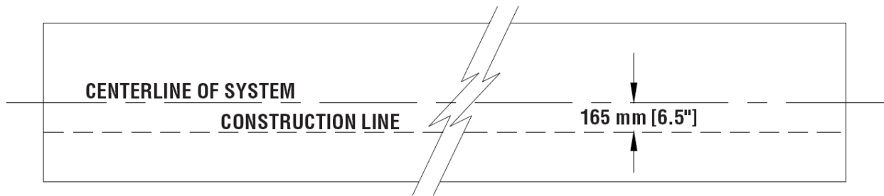
Figure 47 (Top view of concrete foundation)
