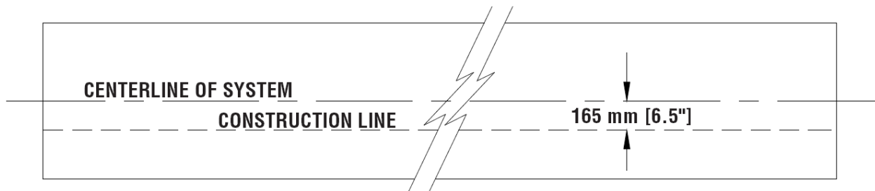
Figure 15 (Top view of concrete pad) Locating Construction Line
