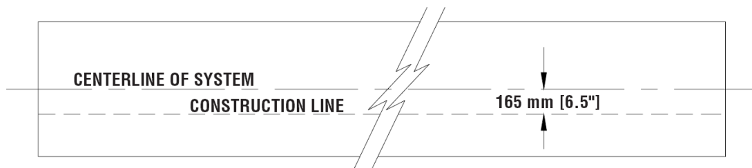
Figure 49 (Top view of Foundation) Locating Construction Line
