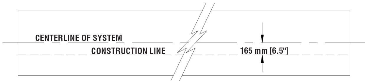
Figure 44 (Top view of Concrete Pad) Locating Construction Line
