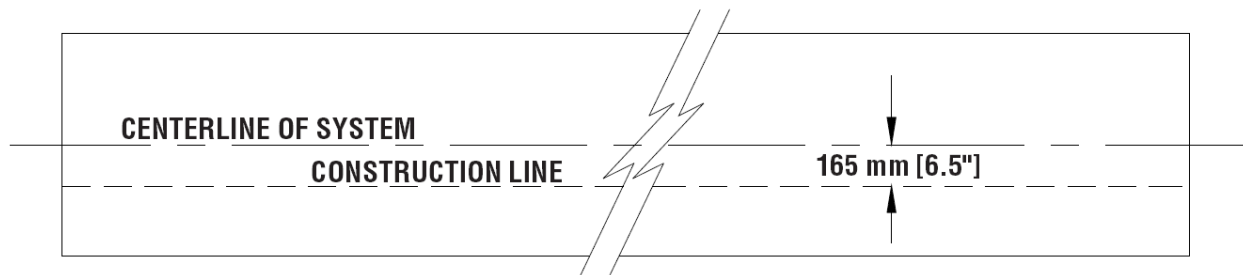
Figure 12 (Top view of concrete pad) Locating Construction Line
