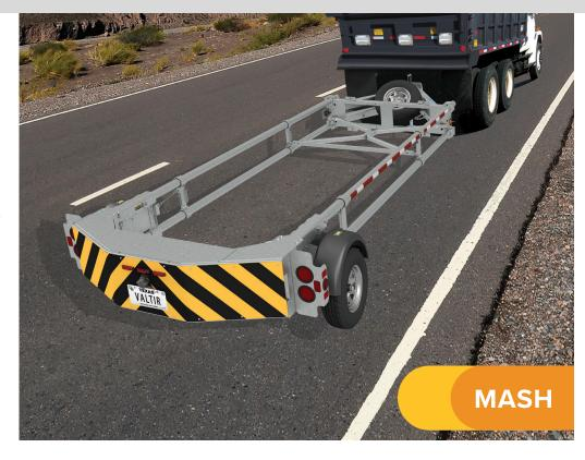
The SMT® is a trailer mounted attenuator for use on stationary or moving shadow support vehicles. It is tested to the Manual for Assessing Safety Hardware (MASH) Test Level 3. The system is comprised of two lightweight aluminum cartridges contained in a steel support frame and heavy duty Torflex® axle and wheels. The SMT® is designed to help absorb rear-end impacts at speeds up to 62 mph (100 km/h) when impacted within MASH crash test standards.\*
