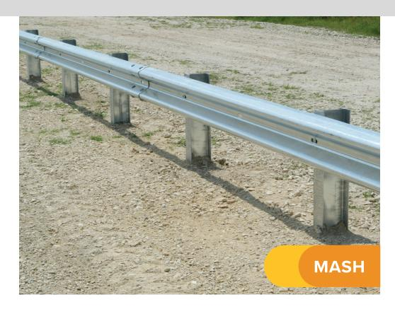
The TGS™ is a 31" high W-Beam, no blockout system. The Standard Strong Line Posts are spaced at 6' 3" with splices either on the posts or between the posts. The TGS™ is tested to both NCHRP Report 350 Test Level 3 and MASH Test Level 3.
