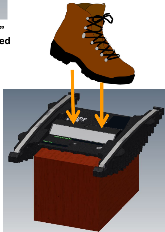
Figure 7 - Placing the Reflector onto the Guide Lite® Marker Body with the marker body center section fully supported by a wood block or similar object.
