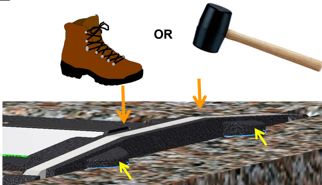
Figure 9 - Ensure that all four leveling tabs are contacting the road surface. (adhesive not shown for clarity)
